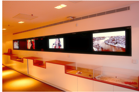
In this installation, the surface of shelves in front of screens might reflect the audio from speakers slightly
